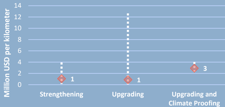
Average unit cost of upgrading roads in Asia, in million USD per kilometer
